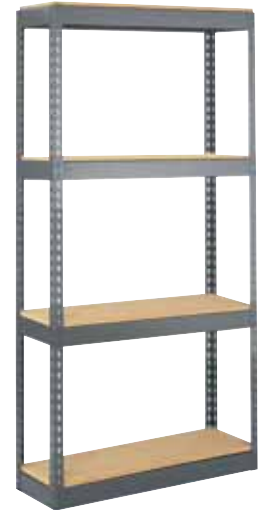
4 Heavy Rivet Angle Posts with Double Rivet Angle beams at all levels - with particle board shelving
